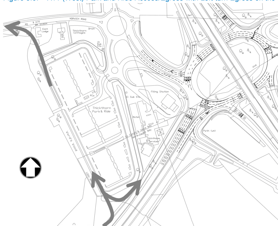
Figure 5.6: A11 (West) Park and Ride Access/Egress with Left-turn Egress on the B1172
